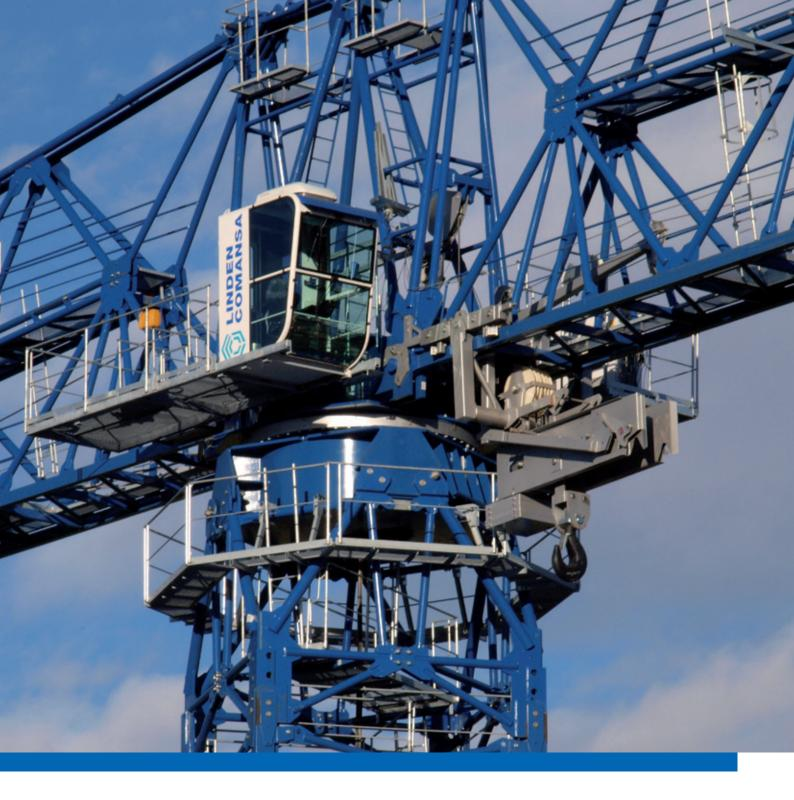
Flat-Top tower cranes with maximum loads from 32 to 90 tonnes (70,550 to 198,410 lb)
